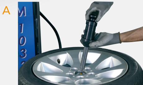
INSERT THE HANDLE WITH THE CLAMPING CONE
