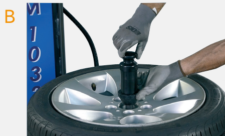
POSITIONING HANDLE WITH CONE ON THE RIM
